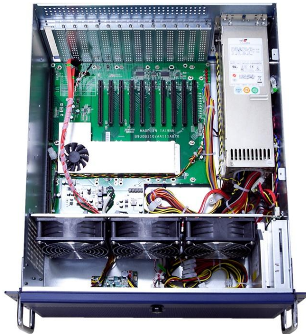
Figure 7 – Portwell's M9020B 4U rackmount chassis offers sufficient cooling and dual redundant 950W power supplies
